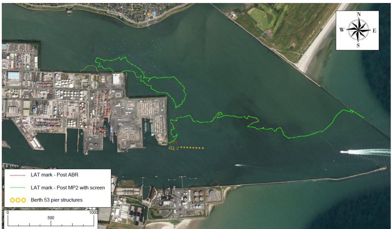
Figure 12-45: Position of the Lowest Astronomical Tide mark post ABR (red line) and post MP2 Project with the wash protection structure included (green line)
