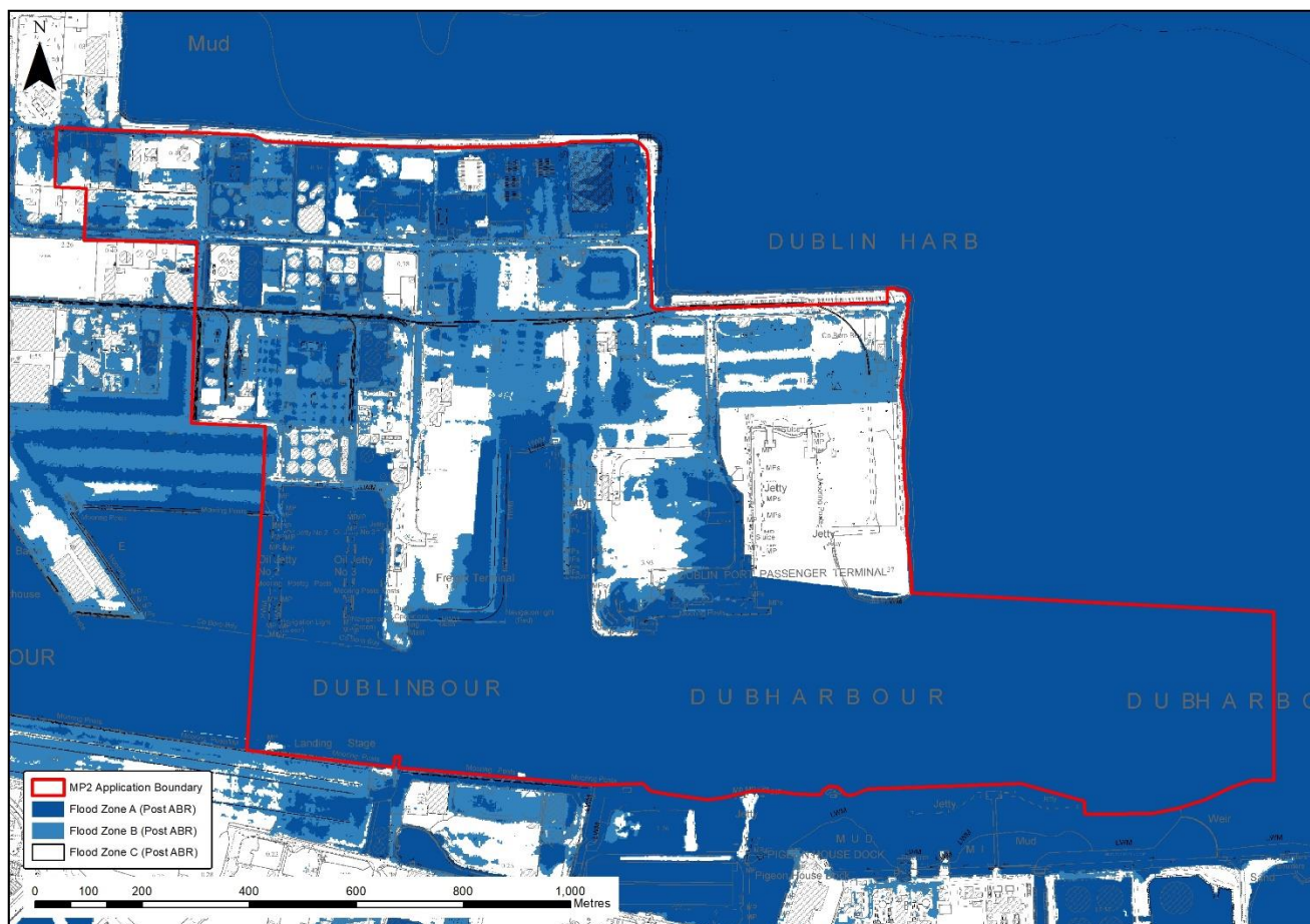
Figure 9-27: Extent of Flood Zones (Post ABR Project)
